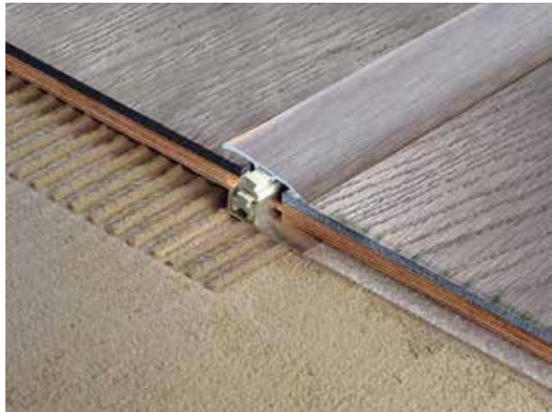
Patented coplanar joint profile. The innovative, ingenious clip system in Resinil (thermoplastic synthetic resin) allows, by simple rotation, to compensate level differences of up to 1.5 mm. The system used with (base) CLB40ANF and (clip) CL40P can also join floors with thicknesses varying from 4 to 6 mm. It additionally acts as a movement joint profile, since the internal cavity allows the underlying flooring to move up to  $\pm$  2 mm.
